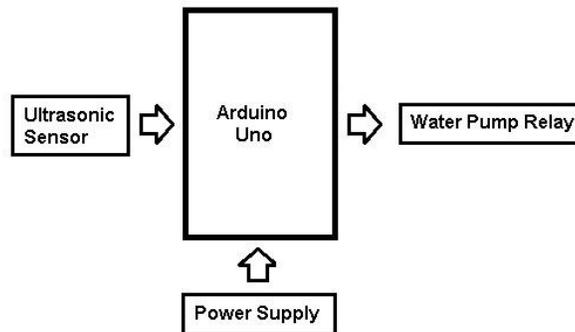
Fig. 3. Schematic Diagram of Hydroponic Nutrient Distribution Control.
